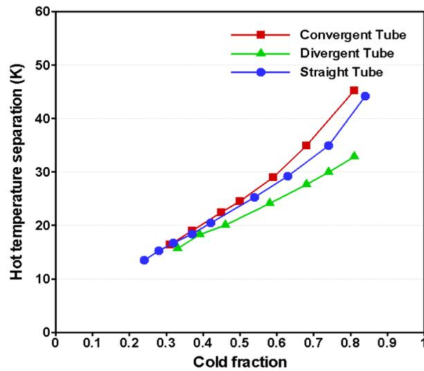
Fig 5: Hot temperature separation in straight and conic tubes
