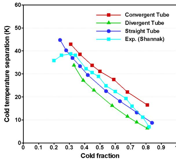
Fig. 4: Cold temperature separation in straight and conic tubes
