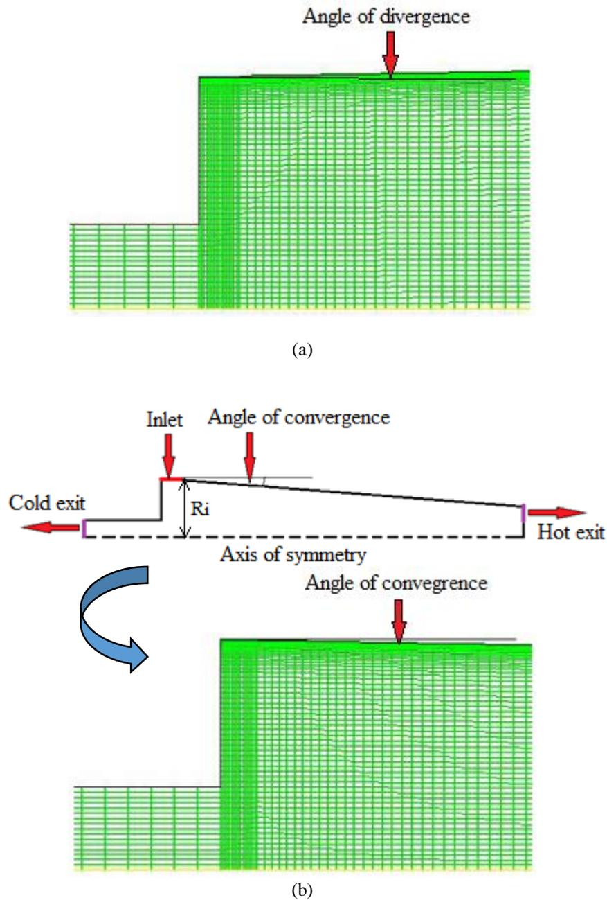
Fig.1: Schematics of vortex tube geometry (a) divergent vortex tube, (b) convergent vortex tube
