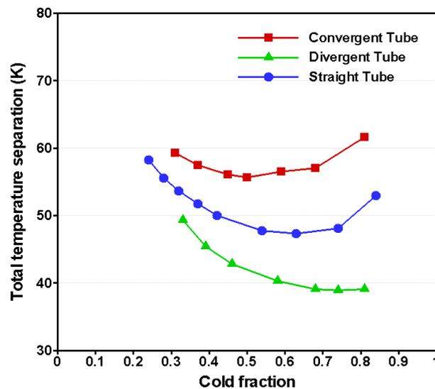
Fig 6: Total temperature separation in straight and conic tubes
