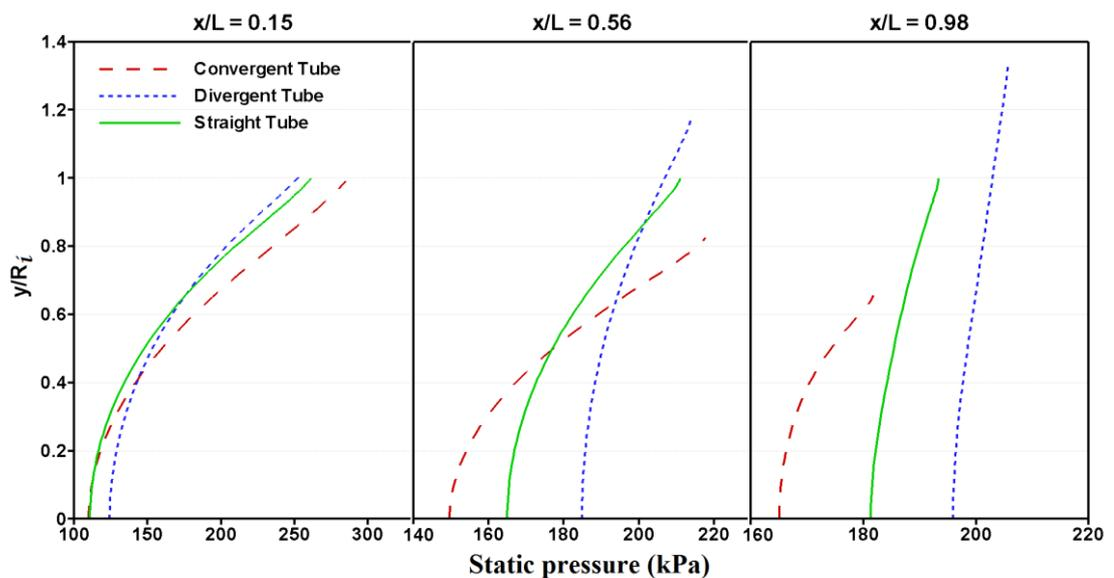
Fig. 3: Radial distribution of static pressure profiles in conic and straight tube,  $\xi = 0.5$
