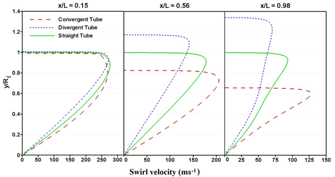
Fig. 2: Radial distribution of swirl velocity profiles in conic and straight tube,  $\xi = 0.5$
